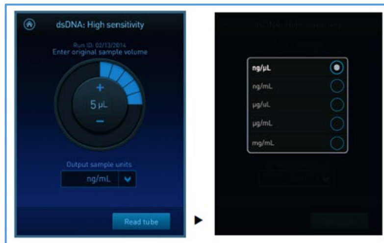
Figure 5: A screenshot of the operation of the Qubit 3.0 Fluorometer for selection of sample volume and unit
